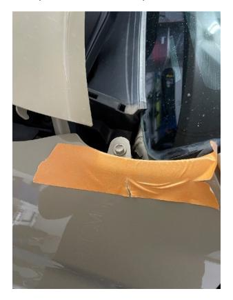
5. Using a 10mm socket carefully remove the fender bolt. Fender may slide out of position, so be mindful where the fender was lined up so body gaps do not change or have clearance issues with hood or doors.
