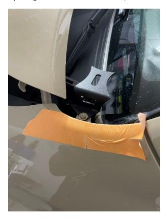
7. Using a marker, grease pen, or pencil mark where the leading edge of the bracket is on the tape. Then install tape to windshield behind ditch light bracket and mark the left and right side of the vertical post. Ensure the inside gap is a little wider so the ditch light wire can be slipped under the cowl corner.
