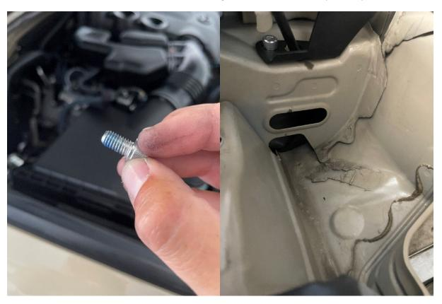
24. The upper hole will be where you fish the nut up onto the fastener. The lower hole is where the socket, extension and ratchet will go up through to tighten down the fastener. (1/4" drive)
