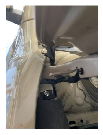
23. Put blue thread locker on the lower ditch light bracket fastener and put into place.
