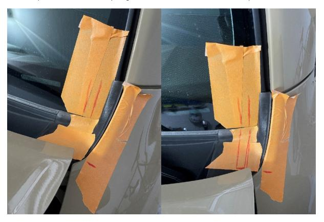
10. Remove cowl corner piece and using a razor blade or saw cut out the boxed section you previously marked.
