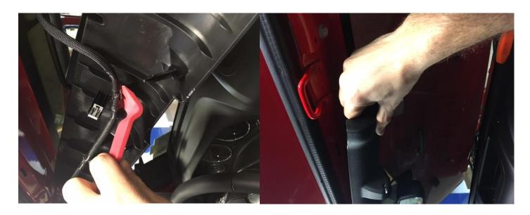
2. Continue running the SP-8100 wiring harness from the engine bay area to the area above the rear view mirror at the TTO Switch Housing
