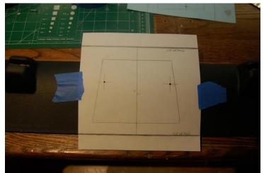
4. Drill two 9/64" holes as indicated with the template. Then drill a ½" hole in the center of the two 9/64" holes using a ½" UNIBIT. This hole is for the wiring to transfer through
