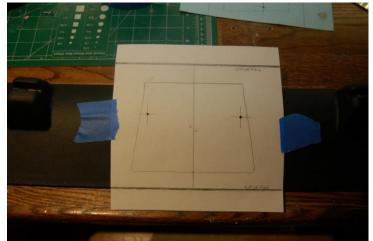
4. Drill two 9/64" holes as indicated with the template. Then drill a ½" hole in the center of the two 9/64" holes using a ½" UNIBIT. This hole is for the wiring to transfer through
