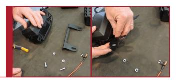
Install the Control Box/Harness by loosening the 10mm bolt on the drivers side fender and remove the 10mm bolt in front of it as shown. Slide the bracket into the 10mm bolt that was loosened and re-insert the bolt on the other. Tighten both bolts to original factory
