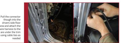
Plug the Control box connector to the switch housing connector, (be sure to hear the "CLICK")
