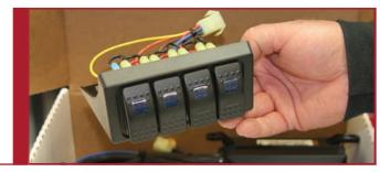
Remove the S-TECH Switch Housing
