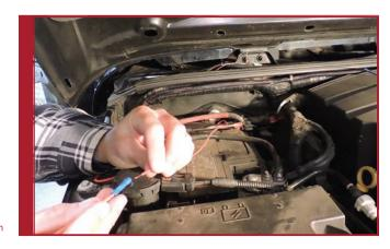
Be sure to note the direction of the fuse tap relative to the Power Distribution Box. NOTE: Front of Jeep.
