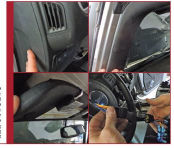
Temporarily remove the Drivers Side Sun Visor and upper/driver side interior trim piece above the rear view mirror while slightly loosening the factory wiring attached to it
