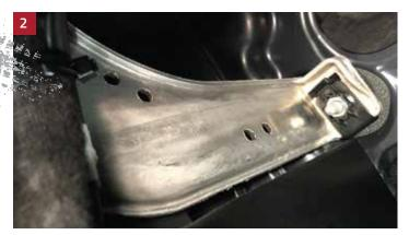
Install the backing plate with the welded 1/4" bolts into the factory upper and lower holes in the metal plate utilizing the holes closest to the firewall.
