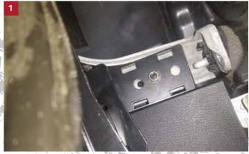
Open the driver's side door and find the metal reinforcement plate above the plastic kick panel.
