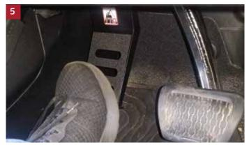
Test fit the dead pedal with your foot to make sure it is located where you want it to be. Make any necessary adjustments and once it is where you like it, tighten the nuts.
