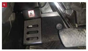
Install the assembled dead pedal over the 1/4" bolt from the backing plate and loosely install 1/4" flat washers, nuts on the bolts.
