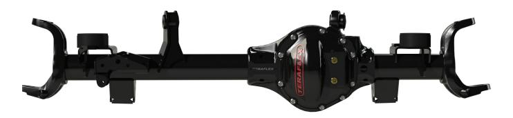
The Tera44 replacement housing is sold as an empty housing to reduce overall cost and is perfect for owners looking to upgrade only the axle housing. Swap over your differential w/R&P, axle shafts, outer knuckles, ball joints, and outer axle assembly (unit bearing, brakes, sensors).
