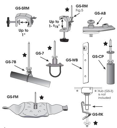
CENTER PIN IS NOT INCLUDED WITH MOUNTING OPTIONS! (use pin that came with GS-1)
