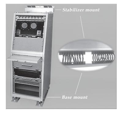
Shown above is an application for shipboard installation. Not only does this arrangement isolate shock and vibration in three axes, but also allows designer/engineers to use COTS equipment rather than the more expensive ruggedized electronic equipment.
