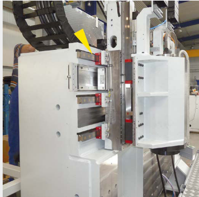
ACE clamping and safety elements maintain a rock-solid hold on the axes in special lathes and secure the predetermined positions both horizontally and vertically
