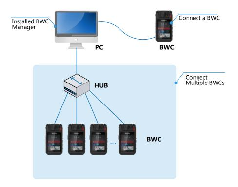
Users only need to install the tool on the PC, and connect BWCs via data cable or hub, then use it to manage BWCs.
