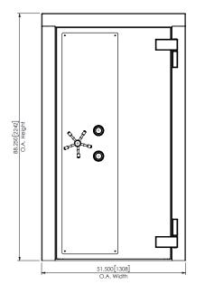
Hamilton's vault doors and frame assembly met the requirements of UL 10C, UL 10B and ULC S104 for a 3-hour fire-resistance rating with hose stream. The Class 1 rating is 30 minute, Class 2 rating 60 minute, & Class 3 rating 120 minute UL security Rating.
