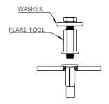
Insert Plus-Nut in the 1/2" drilled hole. Attach washer & flare tool onto 2" bolt and thread into Plus-Nut.
