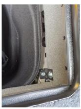
Attach 2 L-brackets to the inside front of the Vault using the  $1/4-20 \times 1$ " hex bolts, 1/4" lock washers, &  $1/4 \times 1$ " washers.
