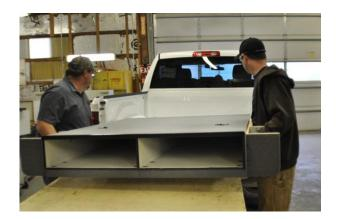
Carefully slide the TruckVault into the cargo area of your vehicle. Position the Vault so it clears the rear hatch or tailgate when closed.
