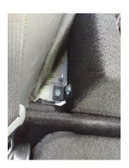
Attach 2 L-brackets to the outside rear of the Vault using the 1/4-20 x 1" hex bolts, 1/4" lock washers, & 1/4 x 1" washers.
