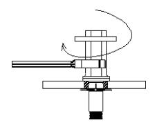
Hold the flare tool with a 9/16" wrench and tighten bolt with impact wrench to collapse insert. Remove bolt, washer, and flare tool.
