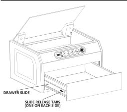
Remove the bottom drawer completely out of the vault by releasing the plastic slider tabs on the inside of the sliders on both side of the drawer.
