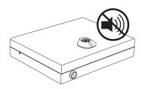
To initiate silent entry mode, hold a programmed finger on the scanner for 5 seconds beyond your fingerprint being accepted. The green indicator ring will turn off and back on, but will not beep, indicating you are now in silent entry mode.
