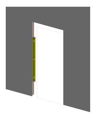
o NOTE: If the RO is not the correct size or out of plumb, a competent contractor may be needed to correct the RO.
