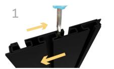
Rails will be nested back-to-back for safe shipping. Be sure to separate before assembling. (It may be necessary to use a screwdriver to separate rails)
