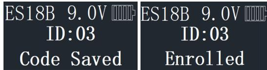
The new code is now enrolled and available to be used to open the lock.
