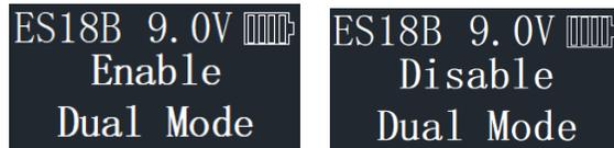
Dual Mode has now been enabled. Two valid codes will be required to open the safe lock system. Open lock by two Users within 60 seconds.
