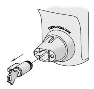
Remove key from cylinder. Hold down the control pin in the end of the cylinder and unscrew the cap.
