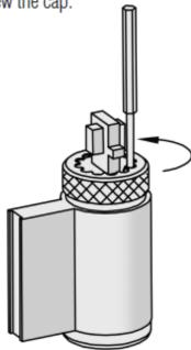
Replace the tailpiece, hold down the control pin and screw the cap fully on without tightening. Ensure control pin projects to lock the cap.
