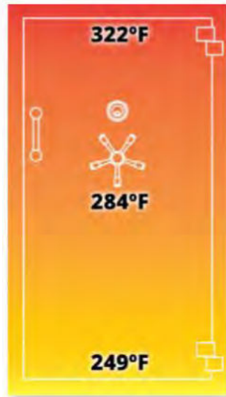
Internal Temperatures When the external temperature is at 1200°F for 2 hours. (paper chars at 450°)
