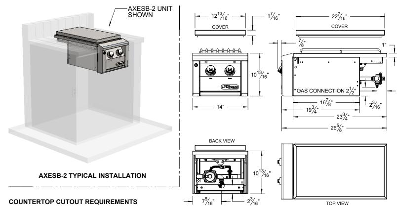
**NOTE**: A GAS LINE IS REQUIRED INSIDE THE COUNTER FOR OPERATION FOR LP-GAS SETUP SEE NOTE AT RIGHT. IT IS RECOMMENDED THAT A FLEXIBLE HOSE IS USED FOR NG-GAS SETUPS
