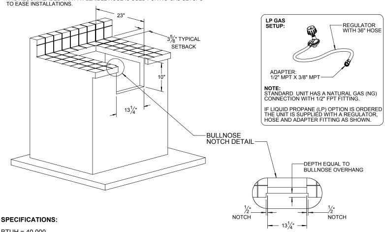
BTUH = 40,000 FUEL = NG @ 5' W.C. OR LP @ 10" W.C. ELECTRICAL POWER = 9 VDC BATTERY GAS CONNECTION = 1/2" NPT (NG) OR 3/8" ODF (LP)
