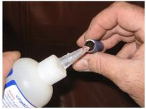
Remove the scuffed brass tube from the assembled barrels and use any familiar method to glue the brass tube into the assembled blanks. Ca glue works great and cures pretty fast. Make sure that you give the glue enough time to cure before you proceed with the next step.
