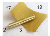
Take the brass tube from your pen kit and prepare it as you would do with any other wooden pen blank. Cut a piece of 3/4 inch blue/ green masking tape (painters tape is also fine) long enough to go around the tube twice.
