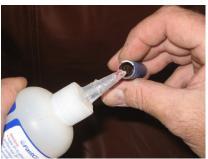
Remove the scuffed brass tube from the assembled puzzle and use any familiar method to glue the brass tube into the assembled puzzle blank. Ca glue works great and cures pretty fast. Make sure that you give the glue enough time to cure before you proceed with the next step.
