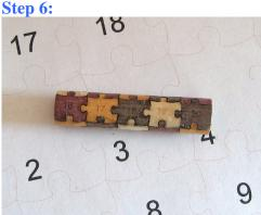
Remove all the masking tape and prepare the trim the ends of the barrel.
