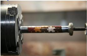
The barrel can now be finished with a finish of your choice. CA glue works great and would provide a great long lasting finish. The pen in this project was finished with CA glue.
