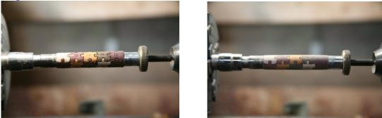
Place the barrel with bushings on the mandrel and place in lathe. Use 180 grit sandpaper to sand the barrel to the desired shape. While sanding place a couple of ( thin ) CA glue drops on the barrel, that would fill all the small gaps in between the puzzle pieces and ensure a great finish product. Use progressively finer sandpaper until you are satisfied with the finish.
