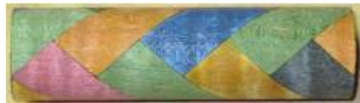
Use thin CA glue over the whole assembly secure all pieces into place before turning the barrel to size.
