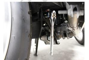
Remove the jack and re-tighten both bolts and nuts with the 17 mm and 19 mm wrenches to medium strength, or if you have a torque wrench then tighten them at 59 N/m (6.0 kgf/m) (44 ft/lb).
