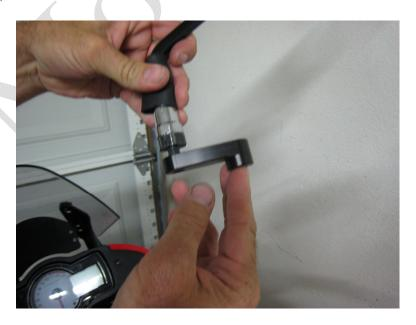
4) Use the **6 mm Allen wrench** to screw the mirror extender to the handle bar with the black hex screw provided.
