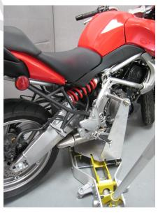
3) Remove the right seat trellis with the 6 mm hex wrench and the 14 mm open wrench.
