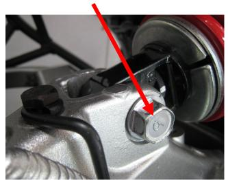
In order to pull the bolt out, you will need to lift the swing arm with one hand and pull the bolt with the other hand.
