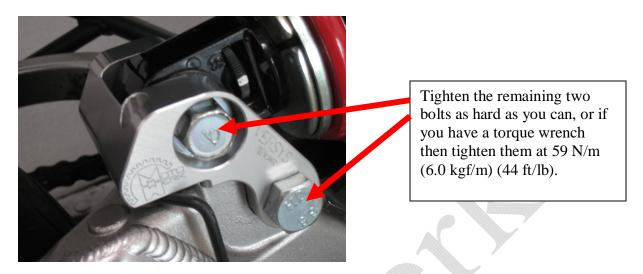
9) Re-install the right seat trellis to the bike with the 6 mm hex wrench and the 14 mm open wrench at medium strength, or if you have a torque wrench then tighten it at 25 N/m (2.5 kgf/m), (18 ft/lb)
