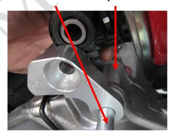
6) Attach the shock absorber to the other hole of the **Main Body** with the original bolt
