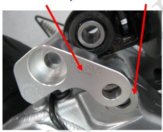
5) Install the M-12 Bolt and the Spacer
