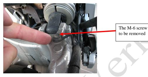
2) Raise the motorcycle so the rear wheel is off the ground. As an example, you can use a motorcycle lift, two car jacks, or upside-down paint buckets that placed under the foot pegs, or a scissor car jack, as shown. "Stable" is the key word. Please take all precautions.
