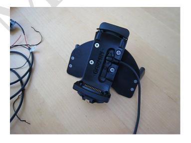
Don't forget to secure the connecting cable per Garmin instructions.
