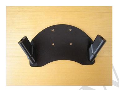
2) Attach the posts to the main plate with the 4 small Phillips screws by putting the screws through the plate from the bottom side and screwing them into the posts
