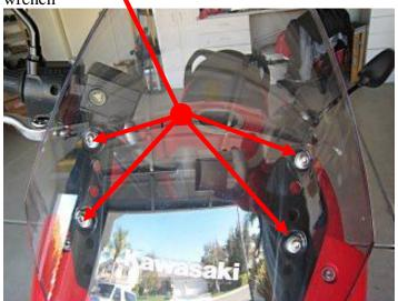
7) Once the windscreen is removed, install the GPS Mount with the 2 large screws to the brackets of the windscreen (from behind).
