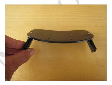
3) Align the Garmin Zumo mount to our GPS Mount, and insert the four screws and locknuts from your Garmin Zumo RAM kit as shown:
