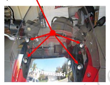
4) Once the windscreen is removed, install the GPS Mount with the 2 large screws to the brackets of the windscreen.
