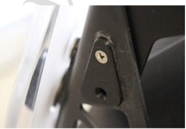
3. Now, screw in the bottom screws through washer and locknut. Adjust the position of the GPS Mount and tighten all screws.
