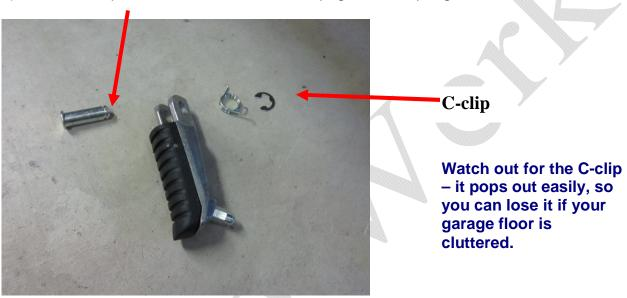
2) Attach the foot peg to the Left Block with the M-12 screw and M-12 locknut provided
