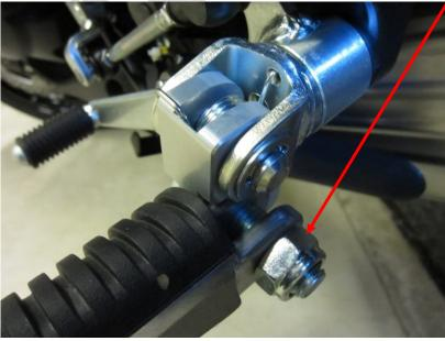
Tighten the M-12 screw and M-12 locknut with two 19 mm wrenches at 25 N/m (2.5 kgf/m), (18 ft/lb) or medium strength.
