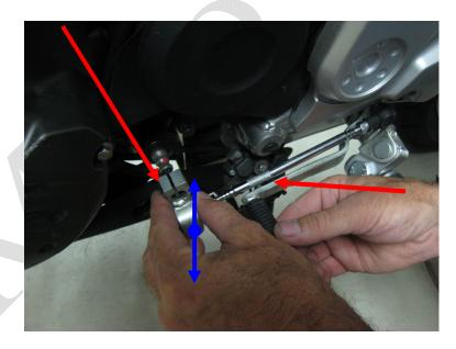
c) Reinstall the screw with a 10 mm wrench
