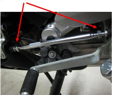
Note: the left (front) nut has a left-handed thread, so to loosen both nuts, please apply the upward motion to the 10 mm wrench in both cases
