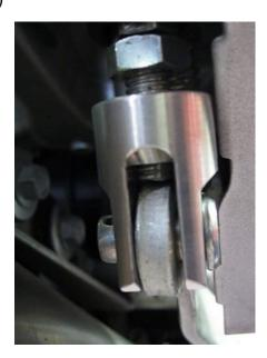
Screw in the brake lever adjustment nut clockwise.
