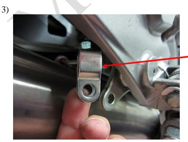
Tilt the cage backwards and unscrew it, together with the inside nut.
