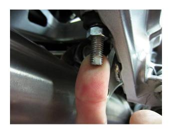
However, if you are still not satisfied with the height of the brake lever, you might have to grind a little off the length of the shaft shown in the photo to the
