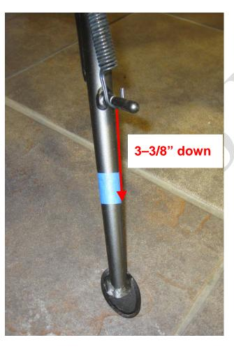
Wrap the masking tape around the kickstand so the bottom of the tape is 3 and 3/8 inches (85 mm) measuring from the bottom of the spring grip peg down, just as shown in the photo.
