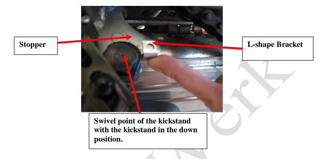
2) With help of another person holding the bike, **swing the kickstand to the upright position**. This way, the kickstand will hold the bracket in place. This is the easiest and the safest way to drill the hole.
