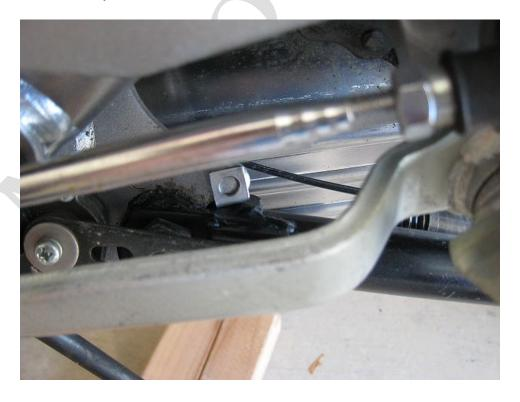
3) Drill the hole in the stopper through the hole in the L-shape Bracket as shown
