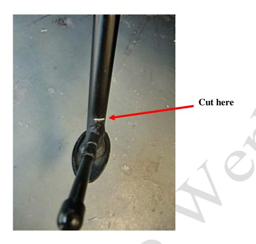
After cutting off the kickstand, please file off the sharp edge of the shortened kickstand's end, so the peg can slide easily into place.
