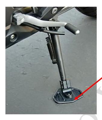
When assembling the flatfoot, please make sure that the pointy tip is aligned correctly with the top peg, as photo shows.
