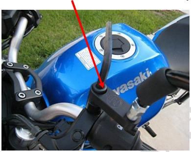
5) Using two **14 mm wrenches** (or one adjustable and one 14 mm wrench) hold the bottom nut and turn the top nut clockwise to loosen it up.
