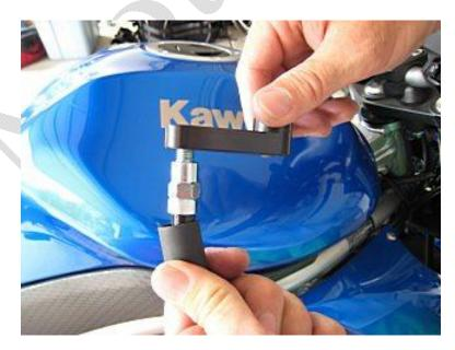
4) Use the **6 mm Allen wrench** (8mm if purchased before 01/13/2010) to screw the mirror extender to the handle bar with the black hex screw provided
