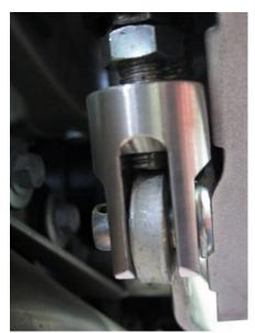
Screw in the brake lever adjustment nut clockwise.
