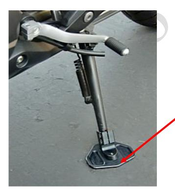
When assembling the flatfoot, please make sure that the pointy tip is aligned correctly with the top peg, as photo shows.
