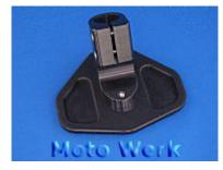
In order to install the flatfoot, you will need to cut off the original kickstand leg. You may use a hacksaw, as shown below. Please **make the cut at 1-1/4**" **above the top of the grip peg**, as shown
