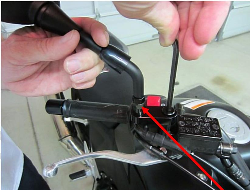
Now, use the 14 mm open wrench to tighten the **lower nut** of the mirror with a **clockwise** motion.
