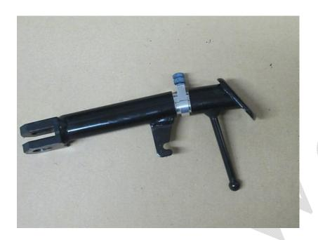
(b) Now, push the kickstand parts together with one hand. Use a 10 mm open wrench to tighten the insert's **screw** with a **clockwise** motion at medium strength. This will cause the insert to expand inside the kickstand. Next, with a **clockwise** motion tighten the **nut** against the insert to lock it into position.
