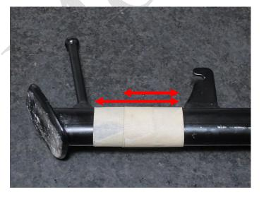
Mark the measured distance with masking tape
