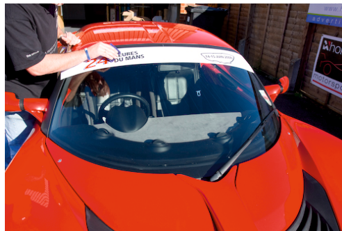
lay the sticker on the windscreen and line the tiny notch, at the top of the sticker, up with the centre-point mark.
