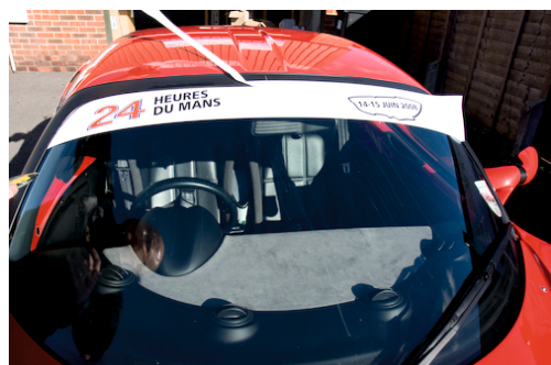
pull away the excess material leaving the sunstrip in place. Squeegee again to make sure all water has been expelled. Allow to dry for 12 hours and test adhesion before driving at speed
