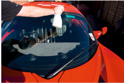
spray the windscreen with a fine mist of water mixed with a couple of drops of fairy liquid
