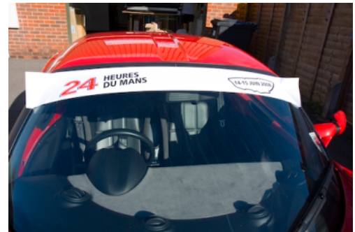
carefully squeegee out the excess water and push the sticker into the edge of the windscreen
