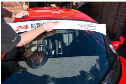
using a sharp blade, very carefully trim away the excess material by running the blade around the windscreen trim
