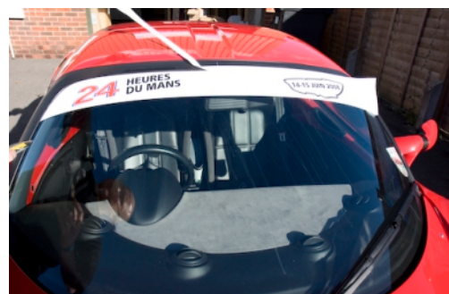
pull away the excess material leaving the sunstrip in place. allow to dry for 12 hours before driving at speed
