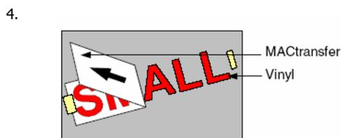
Pull the application tape off at a steady speed, at a cleaving angle of 20 to 45°. Prick any air bubbles (\*) trapped between the vinyl and the substrate.
