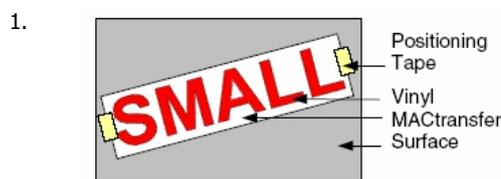
Position the lettering or the logo **WITHOUT REMOVING THE BACKING**, using positioning tape at each end.
