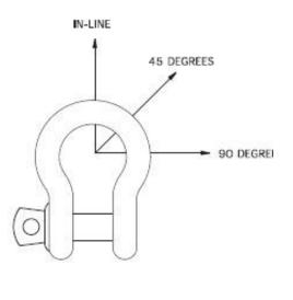
In-line loading is considered to be a load perpendicular to the pin and in the plane of the bow. Load angles in the table are the deviating angles from the in line loads. When using shackles in connection with multi-leg slings, due consideration should be given to the effect of the angle between the legs of the sling. As the angle increases, so does the load in the sling leg and consequently in any shackle attached to that leg.
