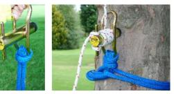
When selecting the best place to mount the device try to locate an area where there is little or no stem taper. If the tree is being removed it may be possible to achieve this by shaping the stem.
