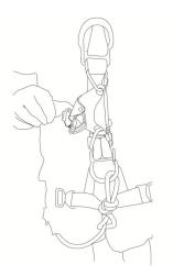
b. When the harness is not in use, always close the cam of the device so objects do not become jammed in the device.
