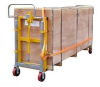
The cabinet being transported must not be left unattended standing on the equipment; it must always be lowered onto the floor. The securing straps may only be opened when the cabinet being transported, or the platforms are standing on the floor.
