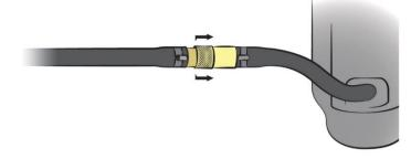
4. To check that the steam hose is securely connected, pull the hose. Ensure the hose is not kinked or restricted.
