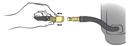
3. Release the barrel of the quick release fitting on the hose, so that it slides into the locked position.
