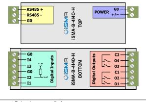
connected together internally All G0 signals are
