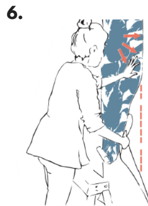
6. Once the panel is secure, reach under & grab the liner. Slowly pull the liner away from the panel while pressing the paper onto the wall & smoothing as you go.
