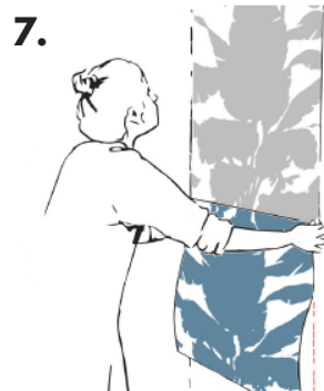
7. Install your next panel below or to the side of your previous panel so they match up and repeat steps 2-6.
