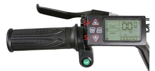
6.**Begin riding carefully**—Hold handlebars and start pedaling on a flat surface, in a low gear (1 or 2), most riders should be able to begin pedaling the bike with pedal assist level 0 or 1. You may also use the throttle to accelerate and maintain your desired speed.
