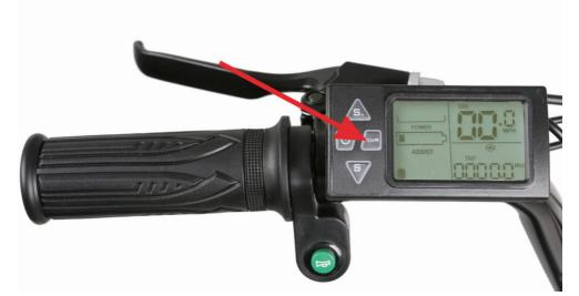
5.**Select the desired level of pedal assistance**—Select the level from 0-3 by pressing "S+" and "S-". Level 1 corresponds to the lowest level of pedal assistance, and level 3 corresponds to the highest level of pedal assistance. Level 0 indicates pedal assistance is inactive. Start in PAS level 0 or 1 and adjust from there.
