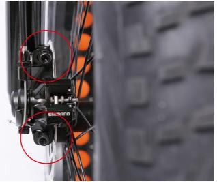
If the pads are still rubbing, we need to do some fine-tuning. Loosen one bolt at a time and adjust until there is a gap on either side of the rotor. Once the pads are not rubbing, fully secure each mounting bolt and the process is complete.
