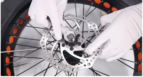
2.Lift the front of the bike and lower the fork onto the wheel axle. **Notice:** The brake rotor should go into the brake caliper in between the brake pads and the axle should enter the fork dropouts fully. The front rotor orientation should be to the left of the fork.
