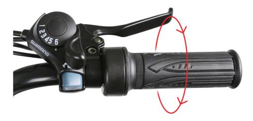
Do not use the throttle while dismounted. Avoid accidental application of the throttle while dismounted; anytime you are moving the bike while dismounted, ensure the bike is powered off to prevent accidental application of the throttle.
