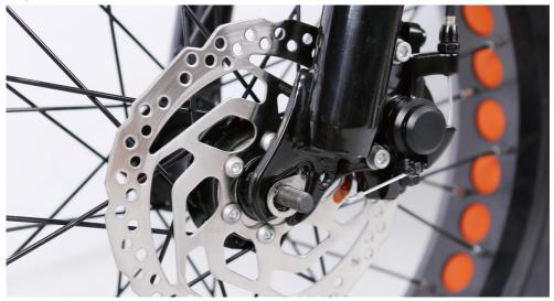
4.Once the lock washers are in place tighten both axle nuts with the supplied double-open end wrench. **Notice:** Before doing the final tight-ening of the axle nuts, make sure the wheel is square and true with the forks.
