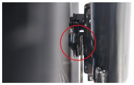
3.After inserting the front axle onto the fork, you will need to line up the axle lock washers (These are the metal washer with a bent tab on one side) with the hole at each fork. **Notice:** These two special fork lock washers keep the wheel from falling off if the axle nuts ever loosen up! Tighten the axle nuts by hand.
