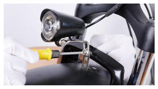
4.Attach the fender mounting arms to the front fork. Ensure the fender is centered and tignten all mounting bolts.
