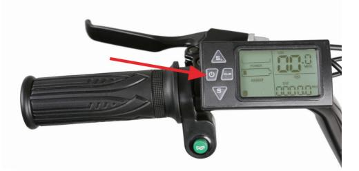
4.**Turn on the headlight** if needed or desired. Once the LCD Display is on, press "CUR" button to turn the headlight on. Press it again to turn the headlight off.
