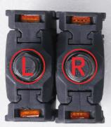
2. The right pedals threaded to tighten by turning clockwise. The left pedals reverse-threaded and tightens counterclockwise. Carefully thread the pedal onto the crank by hand slowly.
