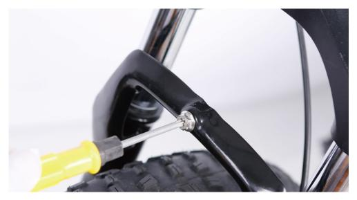
2.Place the fender in position. Pass the front fender mounting point under the front fork arch from the back of the front tire.
