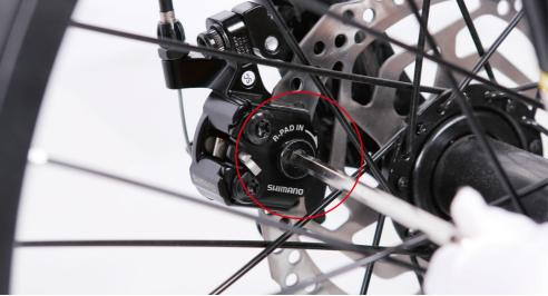
2.Check and adjust the travel at the brake lever at the handlebars. Typically, the pads should feel like they are contacting the rotor at a minimum of 1/2 the lever travel. We will get it by adjusting the brake cable tension.
